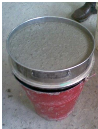
Fig.6 GTM Sieve 5mm Segregation Resistance test (Mixture No. 6)
