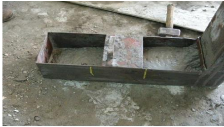
Fig.4. Concrete flowing after opening the gate (Mixture No. 11)
