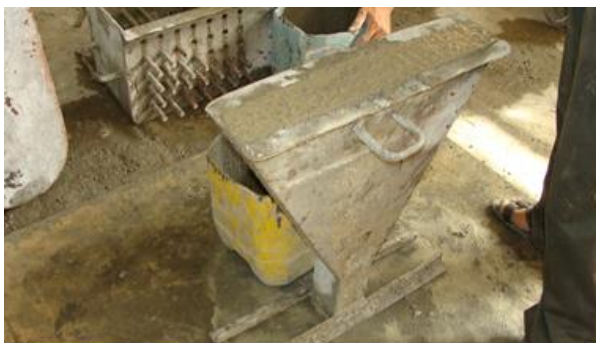
Fig.3. V-Funnel Tst (Mixture No.5)
