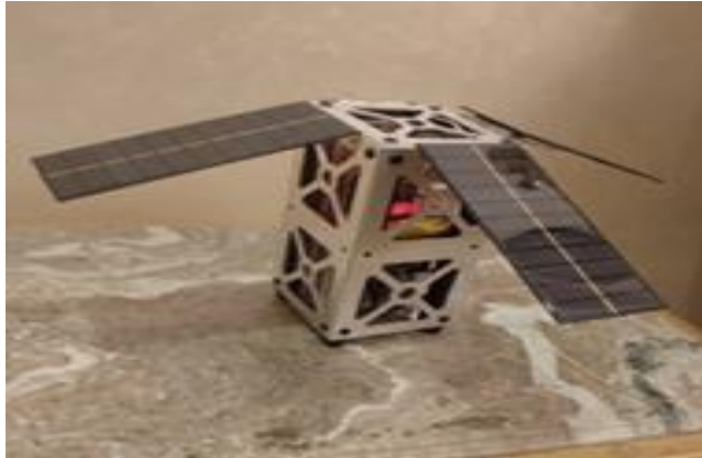
a. The two units cube satellite with solar panels
