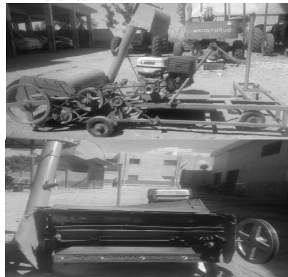
Fig. 2. The innovated packing machine left side and front view.
