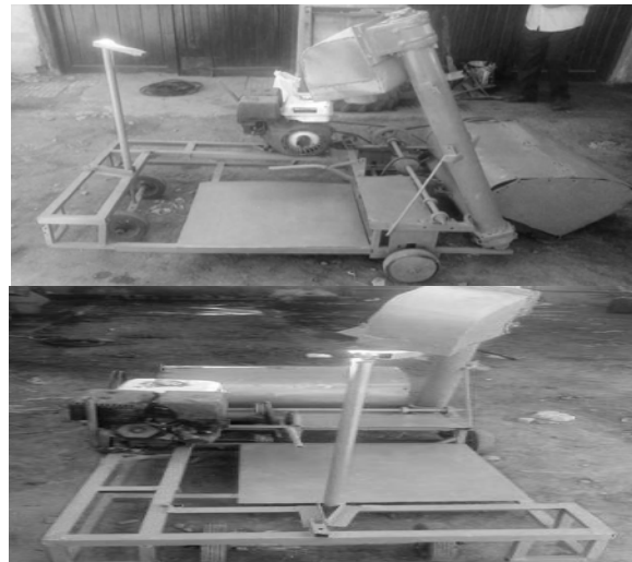
Fig. 1. The innovated packing machine right side and rear view.
