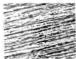
Fig. 12. Optical view showing minimum transfer in steel oil lubricated tests ( \times 100 ).
