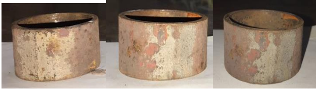
Figures 9a. Three samples of ASME SA-179 pipes before cleaning.
