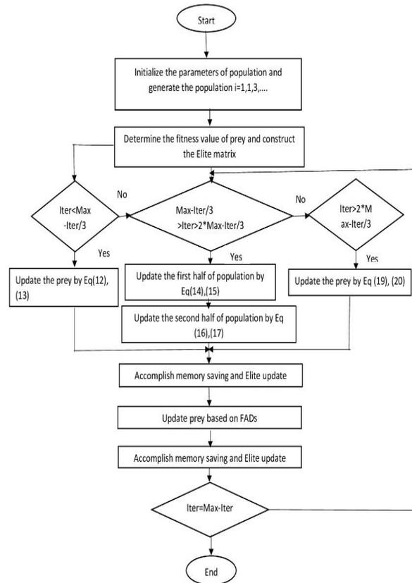
Figure 1 Flow chart of MPO of single MG
