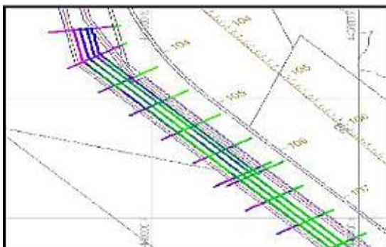
Figure 2: Single Beam Echo Sounder Survey Data
