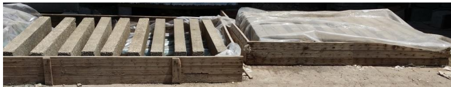
Fig.3: Beams in group G1 placed in boxes outdoors after 300 days
