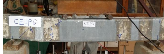
(b) shear failure
