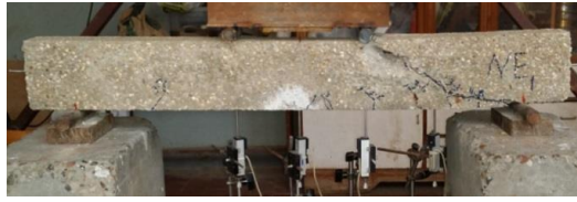
fig.23: shows failure mode of un wrapped
