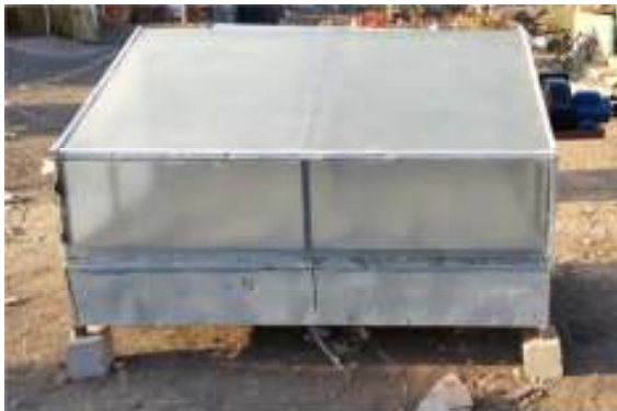
Fig. 2b. Lean-to greenhouse solar dryer.
