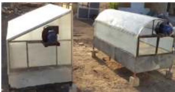
Fig. 3. Modified-Quonset and Lean-to solar dryers used for drying Stevia plants ( Rebaudiana Bertoni ).
