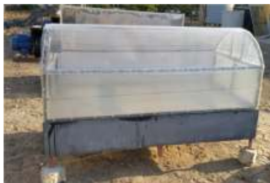
Fig. 1b. Modified-Quonset solar dryer
