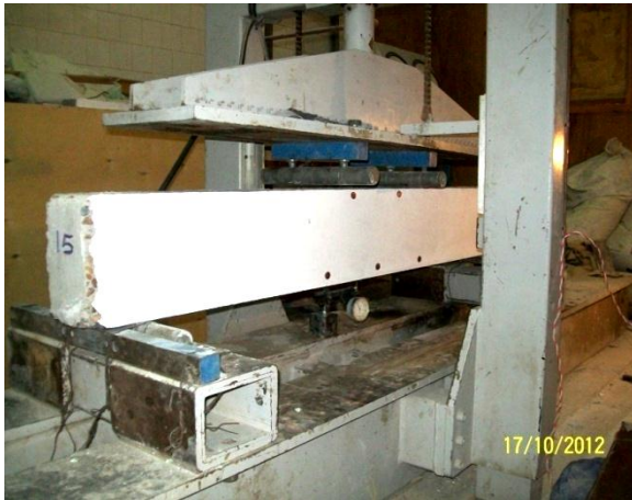
Fig (2): Test setup and position of demec points
