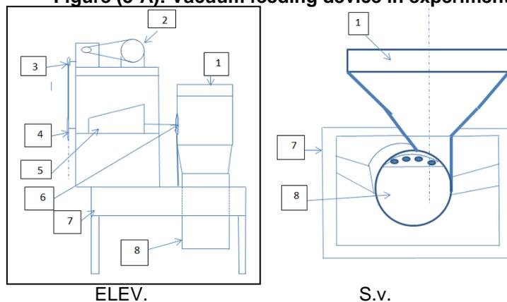
1- Hopper, 2- Motor, 3- Gear16 teeth, 4-Gear48 teeth,
