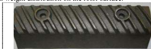
Fig. 2-B: Rasp bar of 15cm
