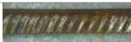
Fig. 2-C: Rasp bar of 30cm
