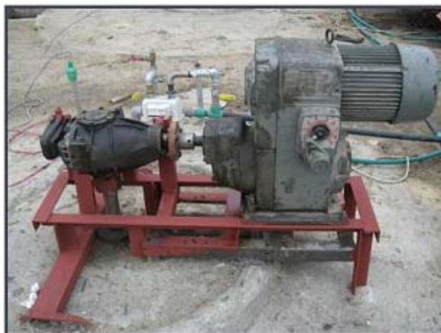
Fig. (2): The variable speed motor connected with the transmission gearbox
